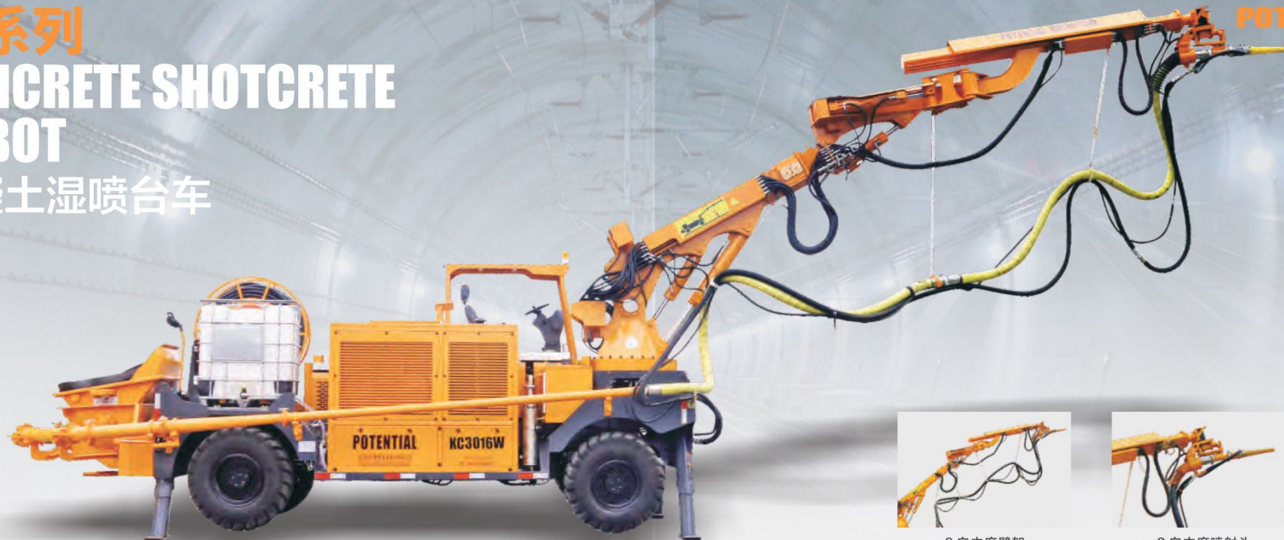
6 自由度臂架 6-PRS Spraying Boom
