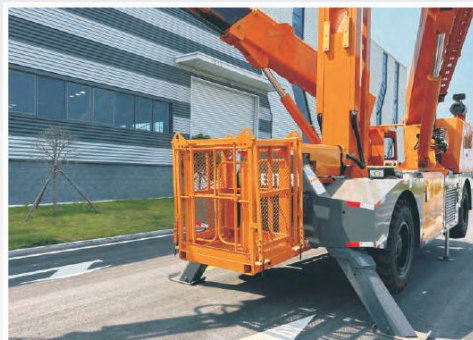
装药平台便携式折叠携带 Portable and foldable loading platform
