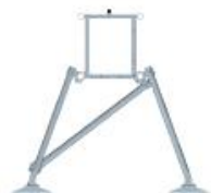
YSC450 附墙架 III mast tie III
