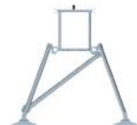
YSC650 附墙架 III mast tie III
